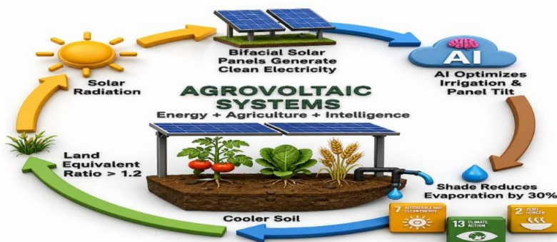
Fig. 1 Operational workflow of Agrivoltaic systems
